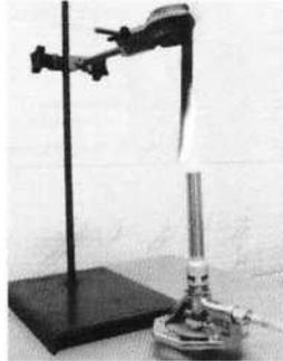
Image 1 View of the test stand used by WCNBOP-PIB in accordance with EN 60695-11-10:2014-02.
